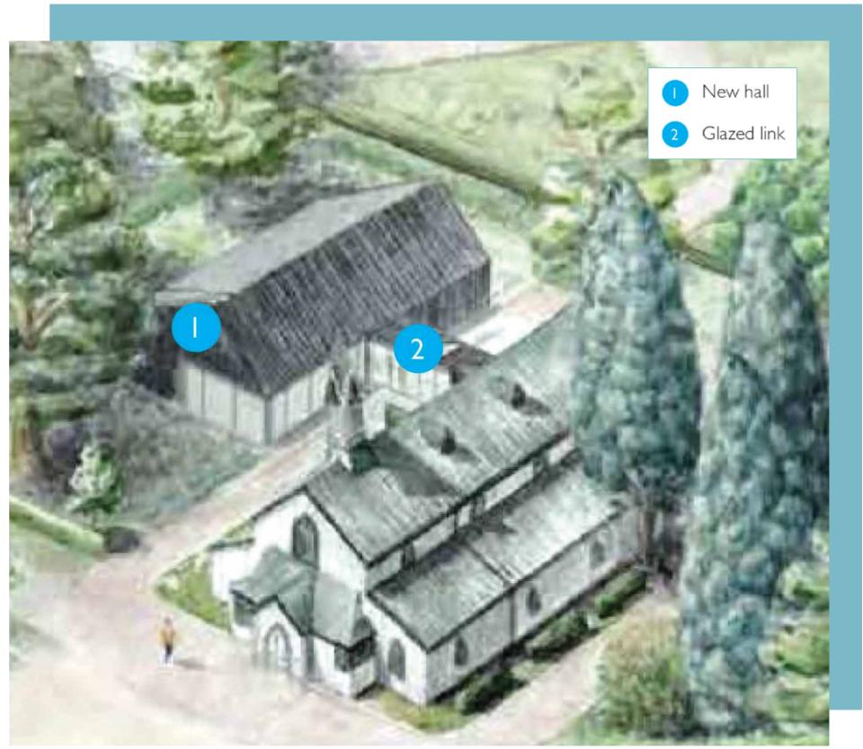
The glazed link attached to the Church has been designed to have as minimal an impact as possible on the fabric of the listed building. The connection through to the church will be achieved by lowering an existing window still to ground level while maintaining the existing width of the current arched window, transforming it into a doorway that will match the adjacent windows.
